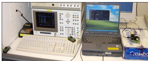
**Figure 9. The power measurement setup**
