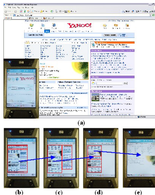
Figure 1: (a) Displaying an original Web page on a desktop computer and a PDA. (b)-(e) Transformed pages of the original page.
