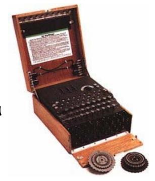
At least once a day the Germans changed the order of the rotors, their starting positions and the plugboard connections. To decipher a message sent using Enigma, you had to work out exactly how all of these had been set.
