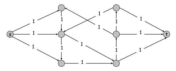
Theorem. Max number edge-disjoint s-t paths equals max flow value.
