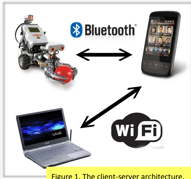
Figure 1. The client-server architecture.
