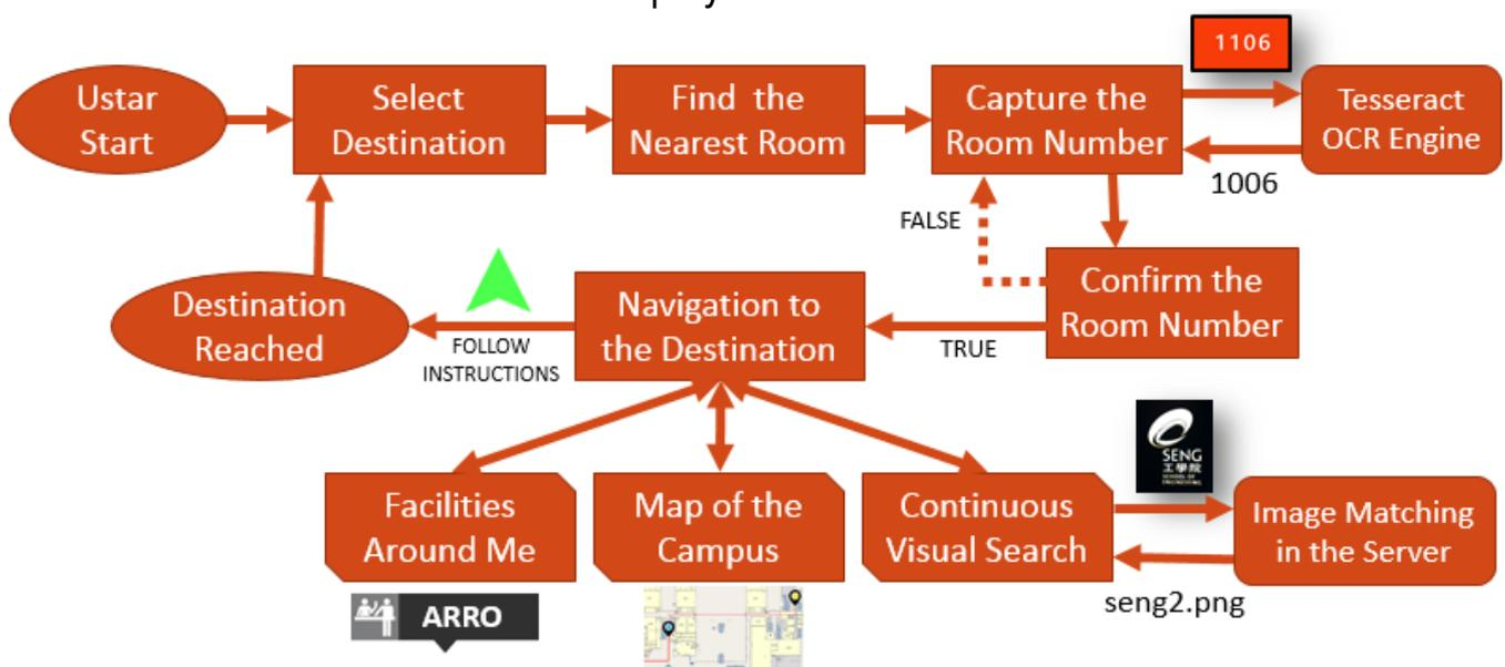
Figure 2. Ustar Run-Through Flow Chart
