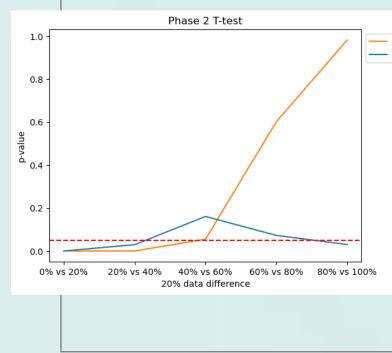
Although using only 20% of the training -  $\frac{1}{100}$  data, there was a significant boost in performance. The T-test proved the MAE difference between 0% to 20% was reliable. It also showed that after 40% data, the MAE difference became insignificant, meaning there was not much performance gained from training extra data after 40%.
