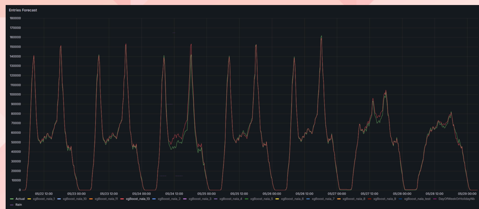
Figure 1: Passenger Flow Analysis (Entry Records) from 22/05/2017 to 29/05/2017 Actual (Green) vs Prediction (Red)
