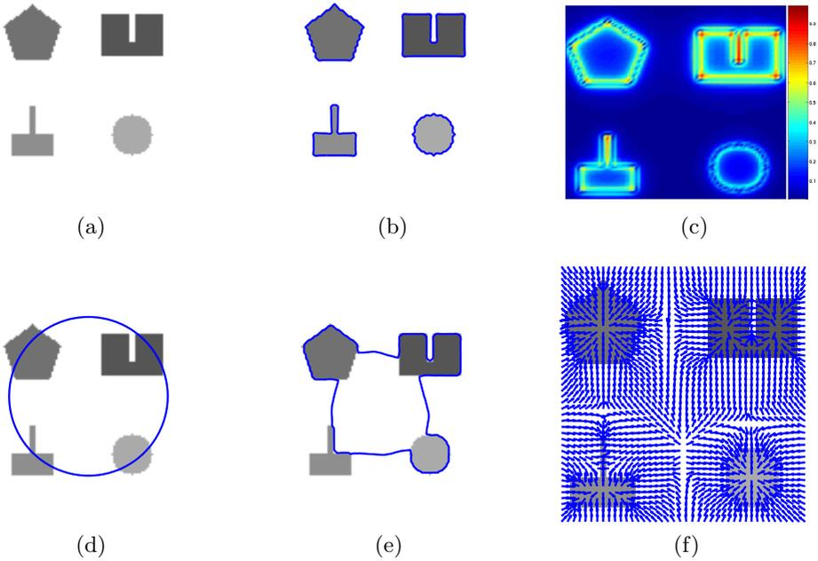
**Fig. 2.** (a) An input image with multiple objects, (b) results obtained using our method, (c) speed field  $v$  of our method (Note that  $\log_2(|v| + 1)$  is shown for better visualization.), (d) initial contour for GVF method, (e) results obtained using the GVF method and (f) GVF force field
