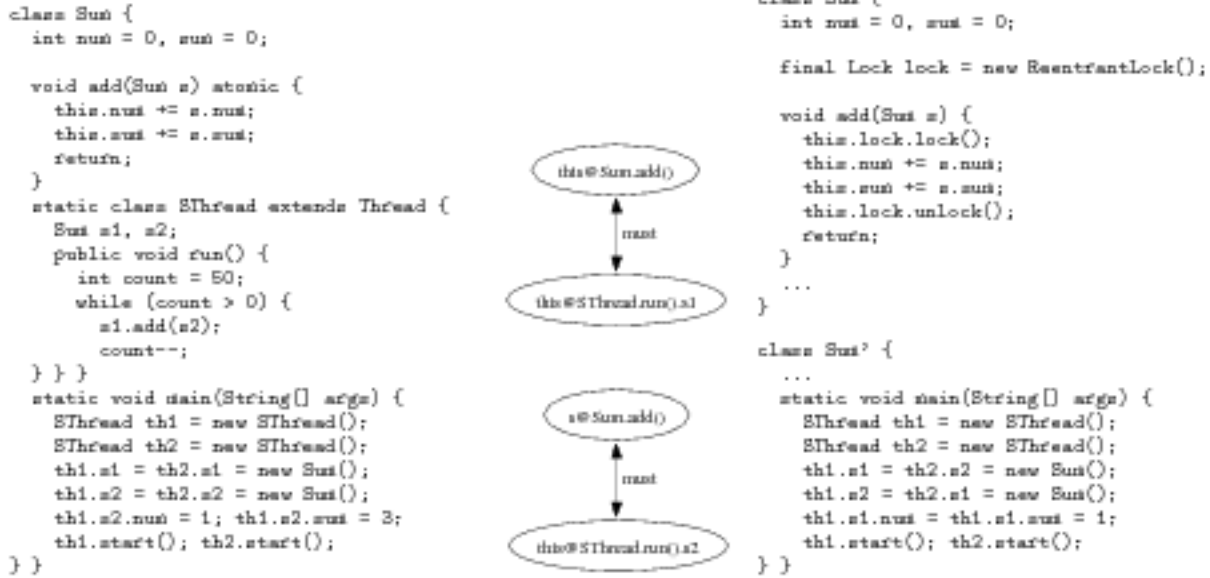
Figure 2. (a) Concurrently executing threads in the Sum module (b) Must-aliases of Sum (c) The rewritten Sum program, protected by locks (d) A similar program, Sum* , in danger of deadlock
