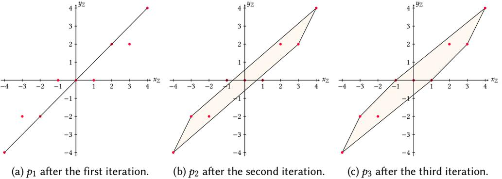
Fig. 3. Major steps for computing the integral polyhedral abstraction of a bit-vector formula  $\varphi$  that has 9 models  $\{(4, 4), (3, 2), (2, 2), (1, 0), (0, 0), (-1, 0), (-2, -2), (-3, -2), (-4, -4)\}$ .
