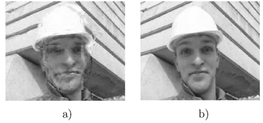
Fig. 8. Subjective comparison of foreman video sequence using pure and hybrid schemes ( p = 0.25, K = 30, \varepsilon_0 = 4\%, \hat{p} = 0.4, n = 45, \text{GoP} = 8, \text{QP} = 3 , and a packet size of 1024 bytes). (a) Pure FEC scheme. (b) Hybrid scheme.
