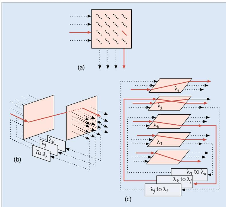
**Figure 3.** Purely optical crossconnects (OXCs): a) 2D using binary (pop-up) mirrors; b) 3D using mirrors with analog control, showing an attached wavelength converter pool; c) multiplane architecture using multiple 2D modules, showing an attached converter pool.
