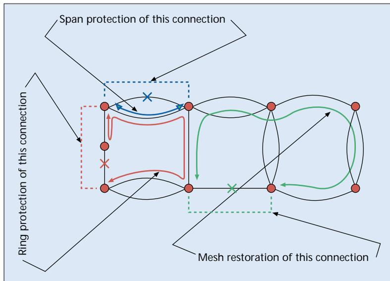
Figure 2. Protection and restoration example: a) span protection, switch to a parallel line; b) ring protection ("BLSR-like" example shown); c) mesh restoration.
