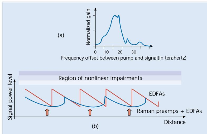
Figure 4. Better amplifiers: a) Raman amplification spectrum; b) curves of optical power level vs. distance showing Erbium amplifiers alone (red) and Raman amplifiers as preamps for EDFAs (blue).
