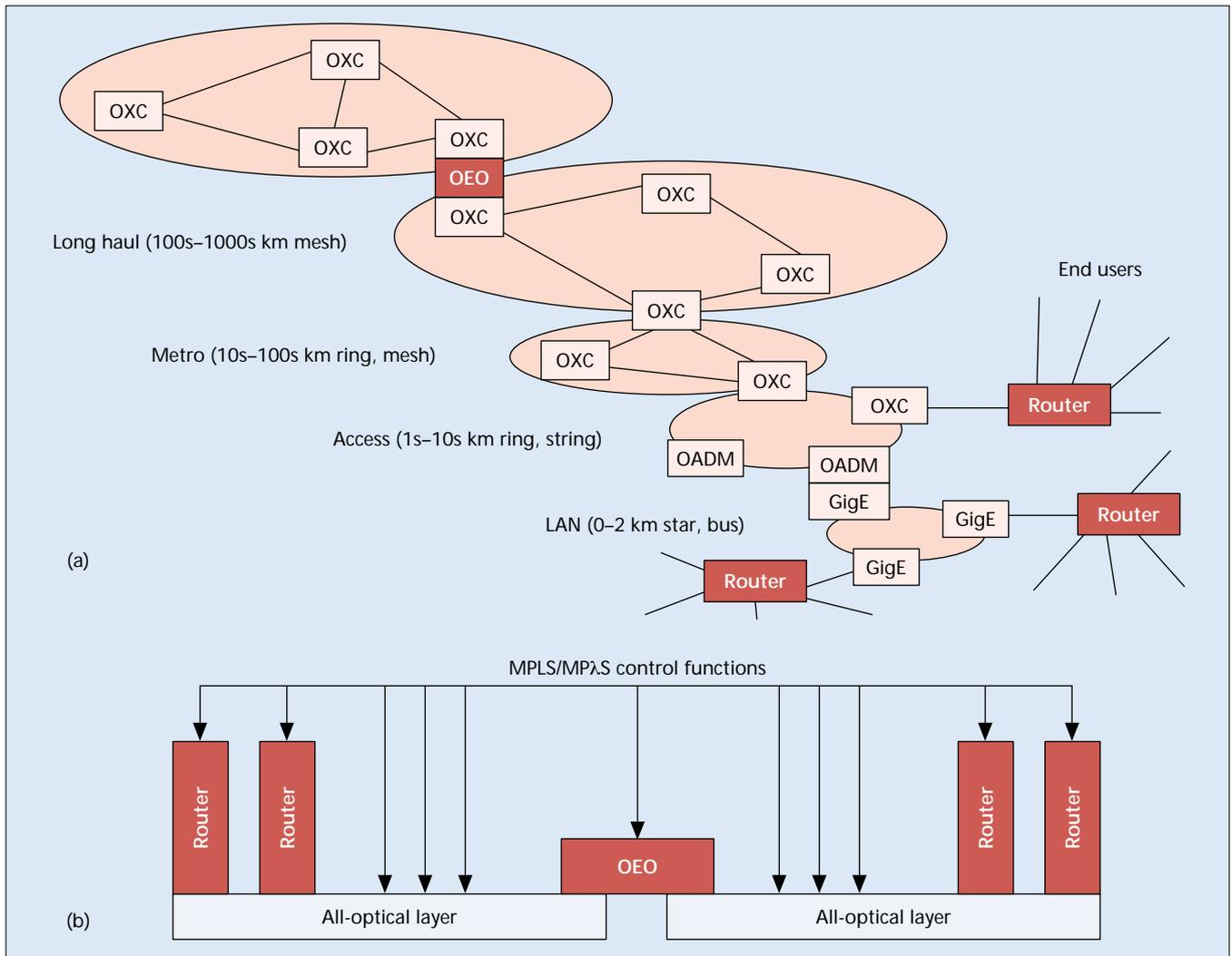
■ **Figure 1.** The optical and IP layers: a) the topology view: islands of all-optical transparency connect to each other via OEO and to users via IP routers; b) the equivalent layer view.
