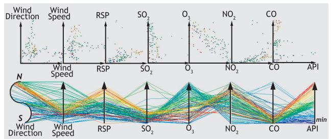
Fig. 8. Enhanced parallel coordinates with S-shape axis to encode wind direction and scatterplot to reveal bi-variate relationship between neighboring axes.
