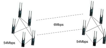
**Figure 17: Clustered MIMO Ad Hoc Networks.** Links within a cluster have high rates, while links across clusters have low rates and hence are the bottleneck. IAC doubles the throughput over these bottleneck links, hence increasing the overall network throughput.
