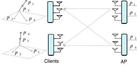
**Figure 7: Four Packets on Downlink.** At the first client, packets  $p_3$  and  $p_4$  are aligned along one dimension, allowing  $p_1$  and  $p_2$  to lie in a two dimensional space and hence be decoded. Similarly, at the second client, packets  $p_1$  and  $p_2$  are aligned, allowing  $p_3$  and  $p_4$  to be decoded.
