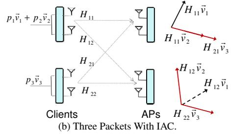
**Figure 4: Three Packets with/without IAC.** In (a), the clients transmit the packets without alignment. The packets combine at the APs along three different vectors and the APs cannot decode any packet. The second case shows how IAC delivers three packets on the uplink. Specifically, two of the three packets are aligned at AP1, allowing AP1 to decode one packet and send it to AP2 on the Ethernet. AP2 uses interference cancellation to subtract the packet and decode the remaining two packets.
