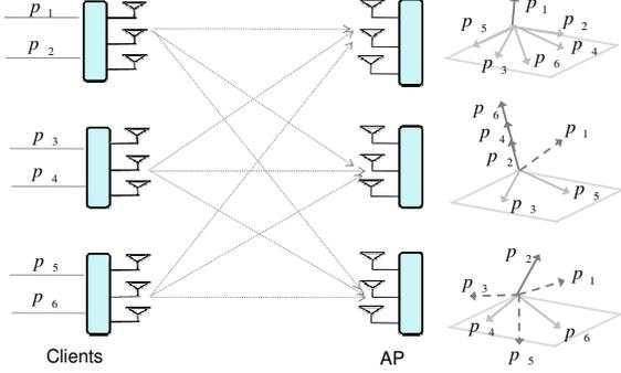
**Figure 8: Six Packets on Uplink.** At AP1, all the packets other than  $p_1$  are aligned on a two dimensional plane, allowing  $p_1$  to be decoded. At AP2,  $p_2, p_4$  and  $p_6$  are aligned along, allowing  $p_3$  and  $p_5$  to be decoded. At AP3, we cancel  $p_1, p_3$  and  $p_5$  leaving  $p_2, p_4$  and  $p_6$  to lie along three different dimensions and be decoded.
