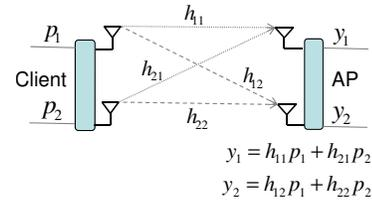
**Figure 1:** Throughput of current MIMO LANs is limited by the number of antennas per node. The  $h_{ij}$ 's refer to known channel coefficients, and the  $p_i$ 's refer to concurrent packets. The client transmits two concurrent packets on its two antennas. The AP receives a different linear combination of the transmitted packets on each antenna, which it solves to obtain the packets.
