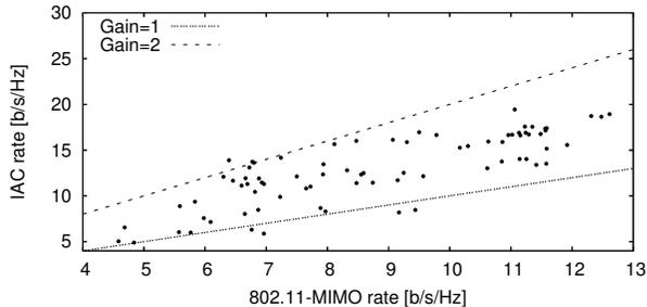
**Figure 12: 2-Client and 2-AP Uplink.** The figure shows a scatter plot of the average rate under IAC and 802.11-MIMO. The rate is measured as bits per second per a Hz of frequency bandwidth. The two lines are for reference; they illustrate the cases of no-gain in transfer rate, i.e., “Gain=1” and a doubling of transfer rate, i.e., “Gain=2”. The figure shows that for the 2-client and 2-AP uplink scenario, on average, IAC increases the transfer rate by 1.5x over 802.11-MIMO.
