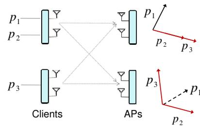
**Figure 2:** IAC Example. AP1 decodes packet  $p_1$  and sends the decoded packet on the Ethernet to AP2 which then performs interference cancellation to subtract  $p_1$ . As a result AP2 can decode  $p_2$  and  $p_3$ .
