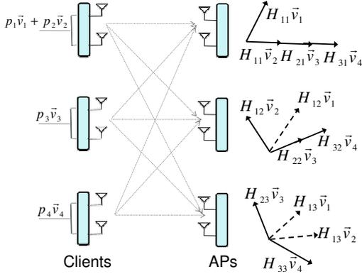
**Figure 5: Four Packets on the Uplink.** In this figure, IAC allows AP1 and AP2 to decode one packet each, and AP3 to decode the two remaining packets. This requires three packets to be aligned at AP1 and two packets at AP2, which can be done by picking appropriate encoding vectors.
