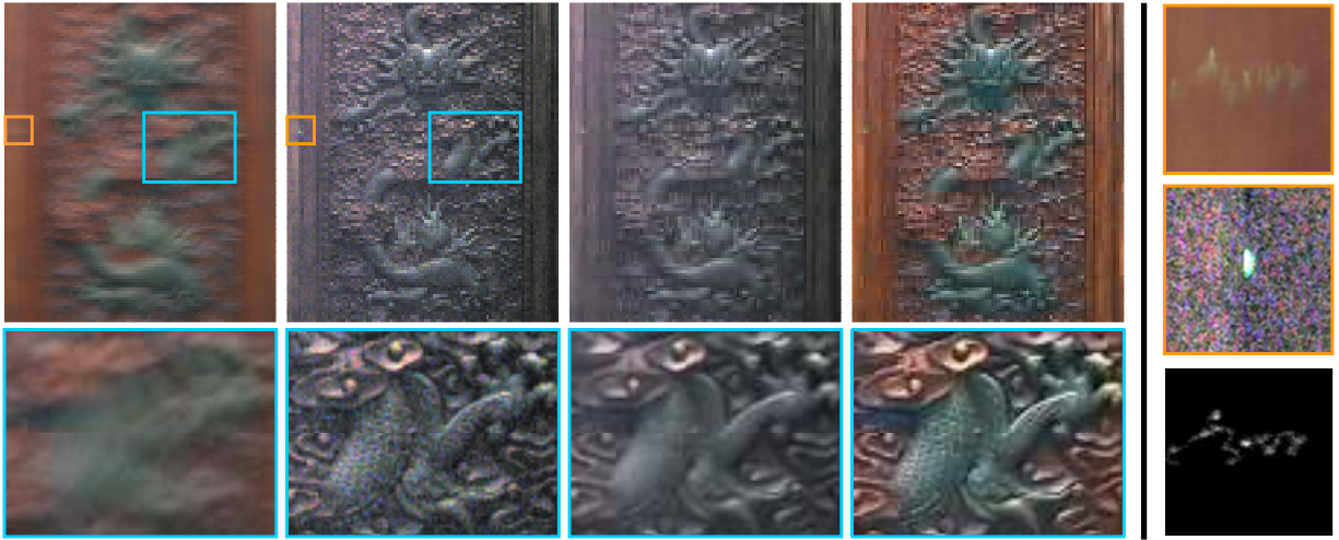
Figure 10: Large kernel. Left: blurred image, noisy image, denoised image, and our result. Top right: two image patches in the light-orange boxes in blurred/noisy images reveal the kernel shape. Note that the highlight point in the noisy patch is an ellipse-like shape. Bottom right: estimated 87 \times 87 kernel.
