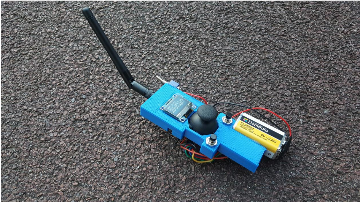
FIGURE 13 3D PRINTED CONTROLLER WITH COMPONENTS, USED FOR THE PROTOTYPE
