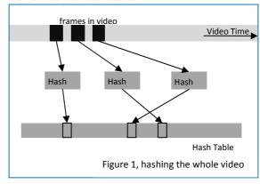
The way we devise the hash value of one frame is: we select four different regions with fixed positions and sizes, computing the gray level of each region. Then we normalize each gray level into [0, levelmax - 1]. Here we choose  $levelmax = 32 = 2^5$ , using 5 bits of space to store one
