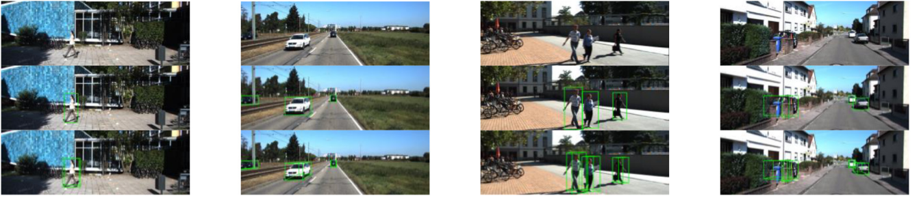
Fig. 6. Visualization results of 2-D box and 3-D box of 3-D object detection. Four RGB images of the KITTI data set are used for visualization. The first line is the RGB original image, the second line is the 2-D box visualization result, and the last line is the 3-D box visualization result.
