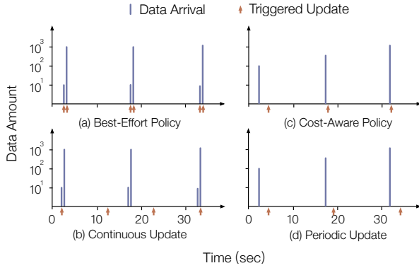
Figure 12: Micro-benchmark of algorithm behaviors. We compare (a) best-effort with (b) continuous update, and (c) cost-aware with (d) periodic update.
