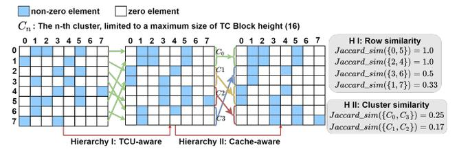
Figure 6. The design of TCU-Cache-Aware reordering. Hierarchy I groups rows into clusters that match the size of TC blocks to improve density. Hierarchy II further groups clusters to enhance L2 cache locality.
