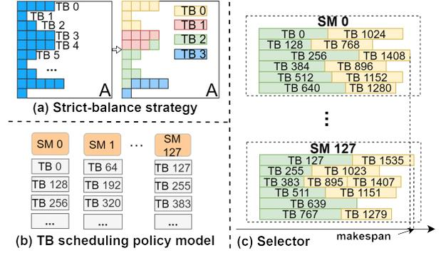
**Figure 10.** Diagram of (a) Strict-balance strategy, (b) thread block (TB) scheduling policy model of RTX4090, and (c) makespan calculation on one SM.
