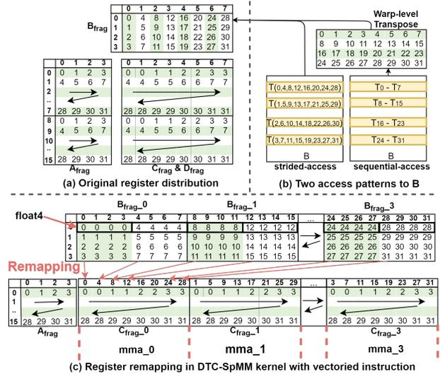
**Figure 8.** (a) The original register distribution of *mma.m16n8k4*, (b) Two thread arrangements to scattered fetch  $B$ , and (c) Register remapping in DTC-SpMM kernel with vectorized memory accesses to  $B$ . 0-31 are lane IDs of threads in a warp.
