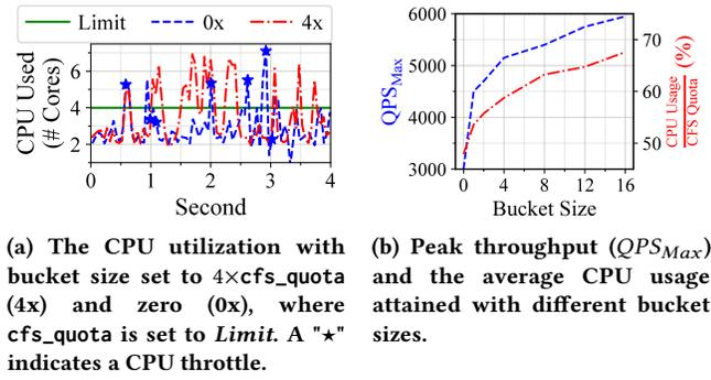
**Figure 13: Running Shore with our burstable CFS controller with varying bucket sizes.**
