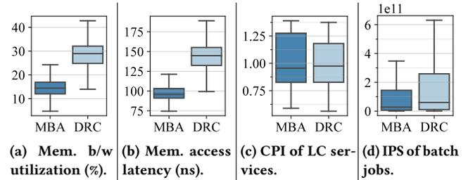
**Figure 18: Performance comparison between MBA and DRC in a production cluster.**
