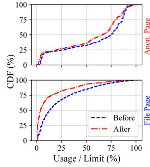
**Figure 8: The anonymous page and file page utilization (usage / memory limit) of all LC instances in a cluster before and after memory reclamation.**
