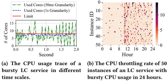
Figure 12: An illustration of CPU jitters.
