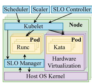
**Figure 2: Illustration of Alibaba's cluster management system.**
