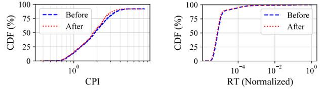
**(a) Cycles per instruction (CPI) of all LC services, before and after memory reclamation. (b) Average response time (RT) of memory-sensitive LC instances (normalized by the longest RT).**
